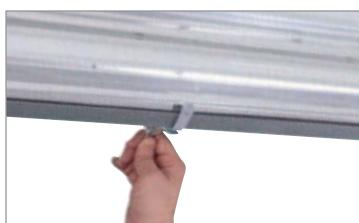
Easy access lamp compartment helps lamp replacement and maintenance operations made quicker and easier. No tools required to open/close latches, to reach inside glass diffuser, all operations done easily by hand.
